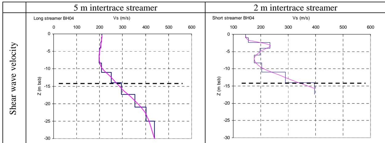
**Figure 5 - Processed data and Shear Wave Velocity Profiles
