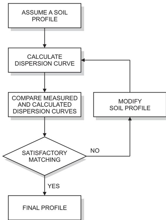
The soil stiffness profile is obtained by means of an iterative inversion process.
