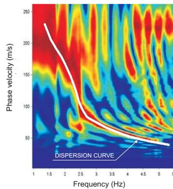
Data is processed by means of Fourier transform and plotted in frequency - velocity space.
