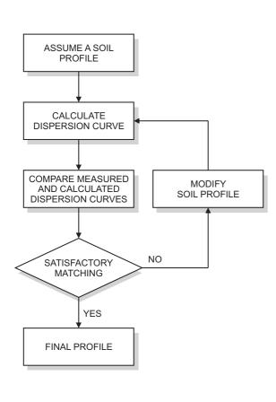
The soil stiffness profile is obtained by means of an iterative inversion process.
